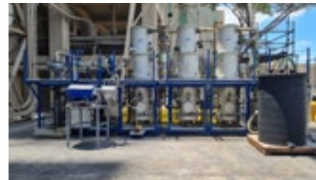
above: Screening unit for optimizing ammonia synthesis
