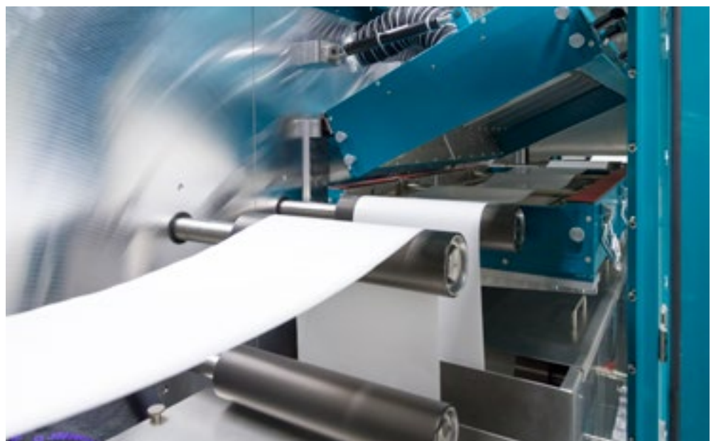
Coatema plant: R2R structuring by means of calender unit
